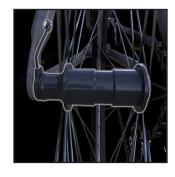
**Dynamo power** generated by the wheel hub: The Dynamo is activated by the hub rotation and generates output power of 3 watts at 6 volts and is appropriate for 16 to 28 inch wheels.
